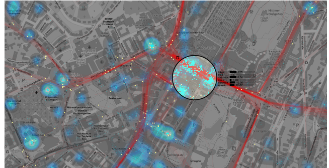
Figure 1: TrajectoryLenses is a Visual Analytics system allowing a user to explore trajectories displayed on a map using a focus-and-context lens. The heatmap shown depicts the end points of movement trajectories to guide the user in exploring the data.
